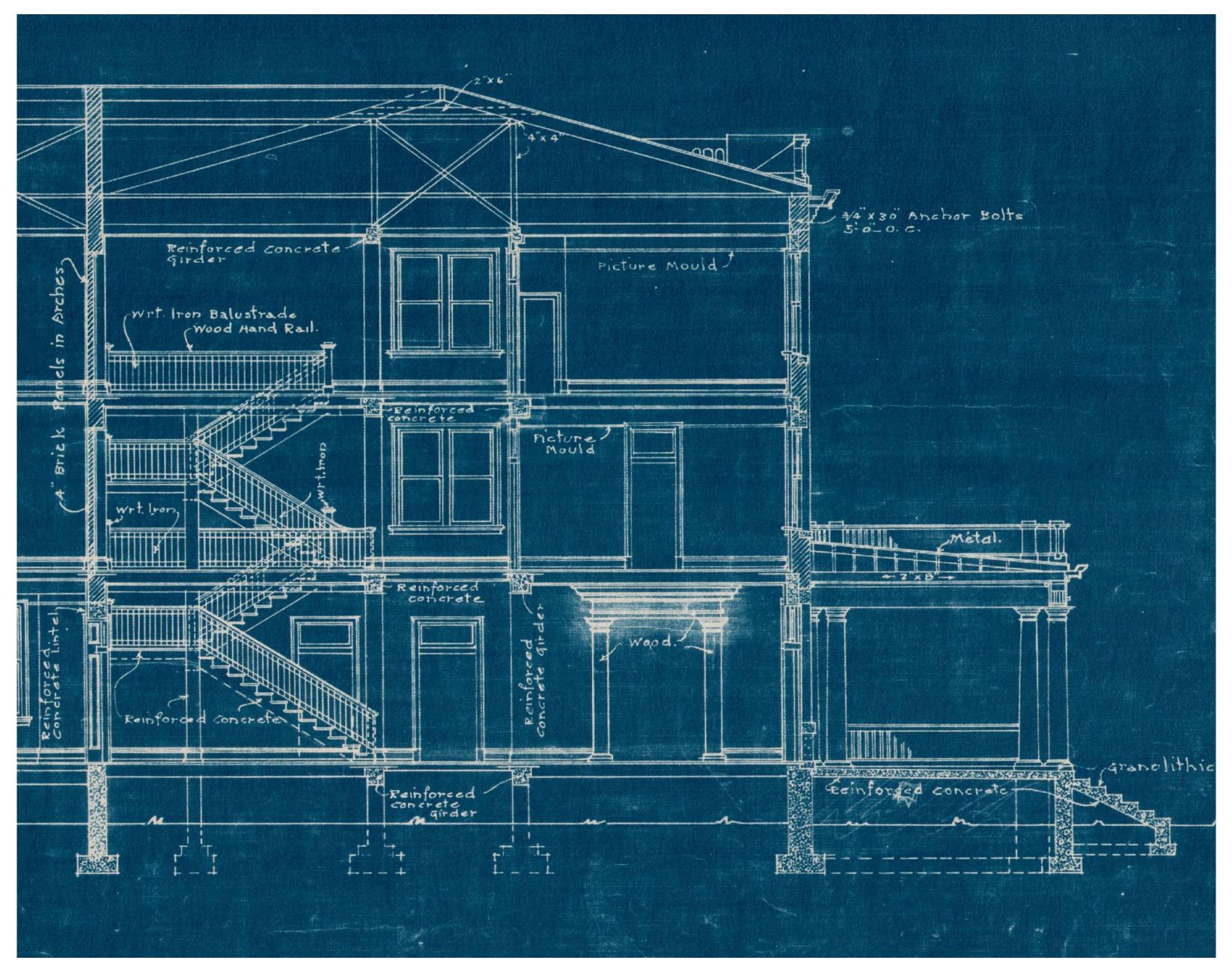
Section of open staircase design for North Wing of Virginia Hall. Notes show original 1914 concrete column design. When built, the stairwell included more modern cast iron columns for support. Image: UMW Office of Facilities
